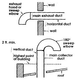
**Do Not** install screening or cap over end of duct.
